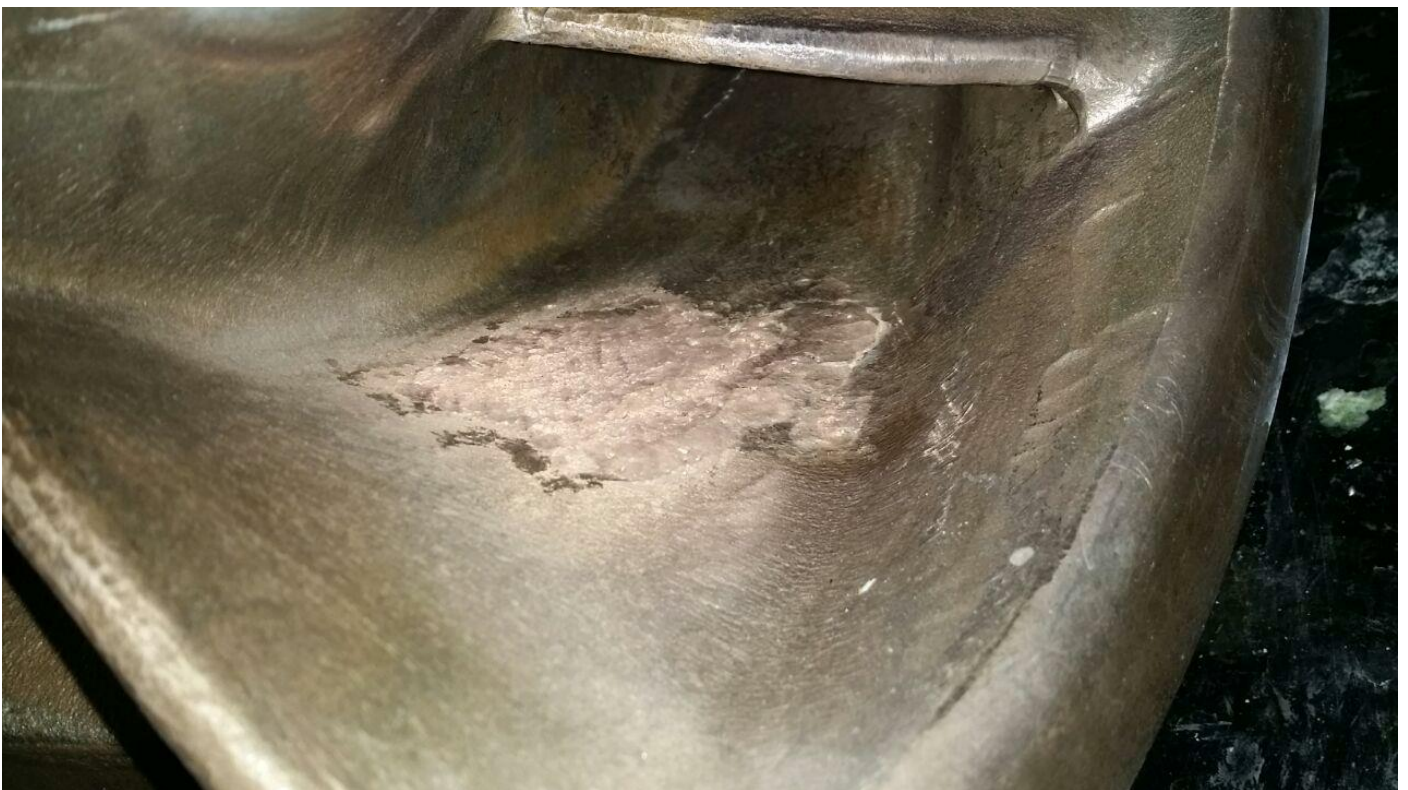
Pitting on impeller (Repaired by Welding)
